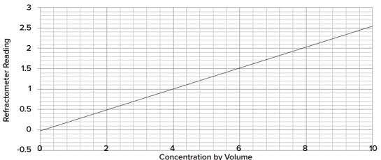
Refractometer Factor: Multiply Refractometer Reading x 3.6
